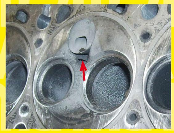
Faults in the injectors flow (incorrect adjustment, dirty hoses, etc.) can cause fuel leaks in the piston chamber.
