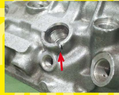
The proper torque given by the OE manufacturer must always be respected. If not, cracks and breakings an affect caps or injector lodgings.
